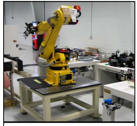
Balancer cell with Fanuc robot.
